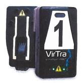
The main module is a clip-on, battery powered, device and is commanded/controlled using a secure wireless Bluetooth link. The wireless link allows freedom of movement inside and outside the simulator and operates up to 50 feet. All RF modules are FCC compliant. The Threat-Fire system comes with the module, a universal voltage battery charger.
